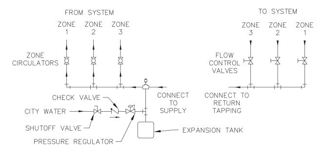
Figure 3.6: Zone Piping with Circulators
